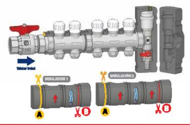
At the outer surface of each insulation, there are embossed slots, indicating the cutting points.
