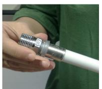
Put the fitting to the pipe and check from the open point of the fitting if the pipe steps to the fitting.
