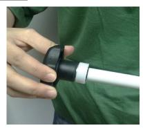
Scrape and calibrate the external and internal surface of the pipe.
