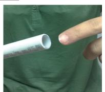
Check the pipe and secure that there are no elements that can destroy the O-rings.
