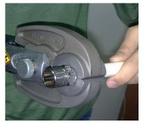
Put the appropriate pressing jaw on the machine and press the fitting, till the point of the jaw connect.
